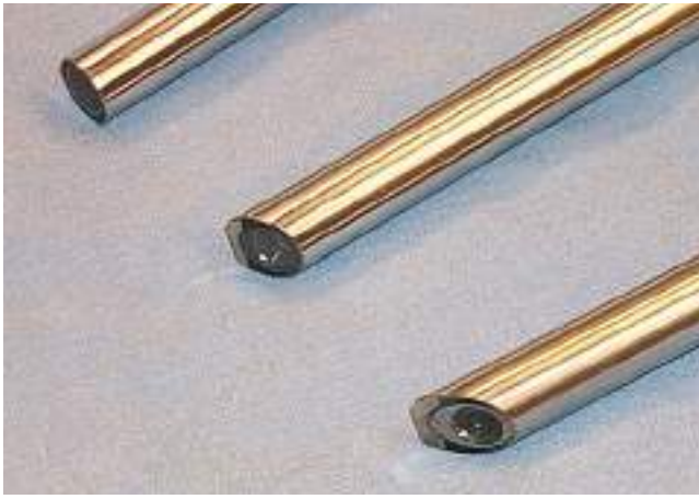
Figure 14-14. The laparoscope tips come in a variety of angled configurations. All laparoscopes have a 70° field of view. A 30°-angled scope enables the surgeon to view this field at a 30° angle to the long axis of the scope.
