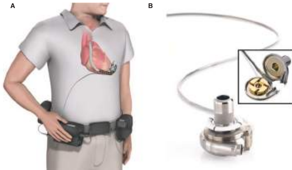
Figure 21-14. The HeartWare HVAD system. A. Both the device controller and batteries are held in a wearable carrying case and connected to the ventricular assist device through the driveline. B. The main component is a centrifugal blood pump, called the HVAD, which is implanted within the pericardium. The only moving part in the device, the impeller, is suspended within the pump using magnets and thrust bearings. Similar to the HeartMate II, it can deliver a flow rate of up to 10 L/min. ( Reproduced with permission of Medtronic, Inc. )
